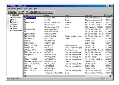
The Printer Panel is the OkiView 32 main display. The display is divided into two smaller panels: the Printer Filters Panel and the Printer Information Panel. The Printer Information Panel, on the right hand side of the main display, shows a list of all the printers currently available for status and configuration. Printer name and status information is detailed to the right of the printer icon.
